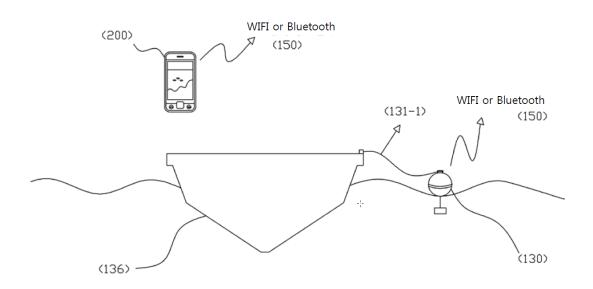
Figure 6 is a block diagram illustrating WIFI or Bluetooth communication 150 between buoy type fish finder 130 and smart phone
