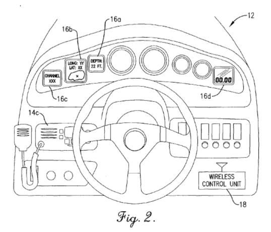
Figure 1 is a block diagram depicting system 10, which is used to wirelessly link electronic marine components. Figure 2 is an isometric view of a helm marine vessel 12 with mounted portions of system 10. Ex. 1007, 2:64–3:3, 3:21–23.
